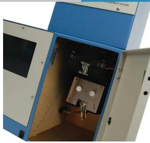
measurements (µg/m³) that account for both non-volatile and volatile PM-10, PM-2.5 and PM-Coarse components. The system's default data output consists of a running 1-hour and 24-hour average mass concentration updated every 6 minutes and on the hour respectively. The monitor computes a 1-hour FDMS base and reference mass concentrations updated every 6 minutes. Users can select additional averaging times from 30 minutes to 23 hours.
