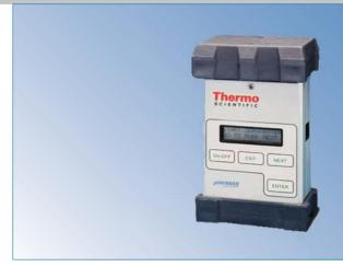
The Thermo Scientific personal DataRAM pDR-1000AN Monitor is a passive sampling, light-scattering nephelometer that measures real-time mass concentrations of dust, smoke, mists, and fumes in industrial as well as other indoor and outdoor environments.
